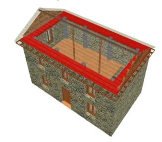
Fig. 14. Ring Beam highlighted in red is installed at the top of the attic wall
