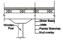
Fig. 4. Intermediate wooden post to floor connections
