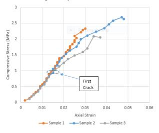
Fig. 21. Compressive stress vs Axial stress
