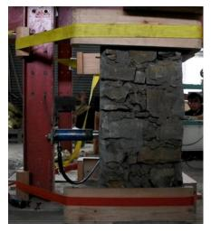
Fig. 23. dowel push out tests setup
