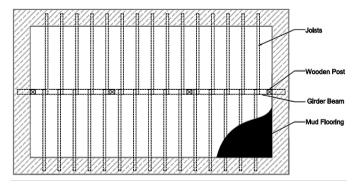
Fig. 6. Floor plan showing joist and Girder beam placements
