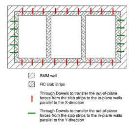
Fig. 18. The red and green lines indicate dowels spaced at 600mm that connects the slab strip to the walls
