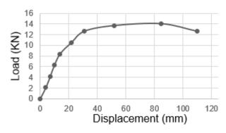
Fig. 22. load displacement curve for push out of dowels
