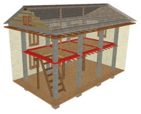
Fig. 17. Slab Strip (indicated in red) connects the diaphragm to the walls as well as interconnecting the strong backs
