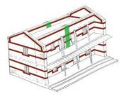
**1.** Belt at eave, lintle/ floor and sill levels on all walls, inside and outside along with a composite column at mid-length, if length exceeds 5m (16'4")..
