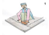
1. Clean the crack with wire brush.
