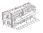
6. Horizontal Containment Reinforcement (CR) wires on all the walls on both the faces anchored to the Vertical CR wires in the vicinity of the cross-links in the clear space between the belts with horizontality maintained with the help of tube-level. <u>No</u> Horizontal CR wires are to be placed on the belts. Wires to continue over the splints and opening encasement.
