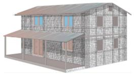
Figure 8: Splint and bandage approach (Source: NRA's Repair and Retrofitting Manual)
