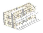
5. Vertical Containment Reinforcement (CR) wires on all the walls on both faces anchored to the walls through cross-links placed between the Corner Splints and Opening Encasement continuous from ground story to the top of attic walls maintaining verticality with plumb bob. No vertical CR wires are to be placed on splints and opening encasement, and are to continue over the belts.
