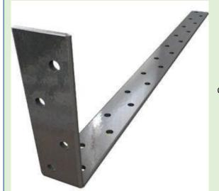
3 mm thick width and depth : 115mmx300mm, M8 of 4 number, (width side) and M8 of 8 numbers depth side face @ 4.5 m at centres
