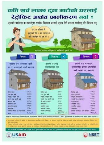
Figure 48: Cost comparison of retrofitting with new construction
