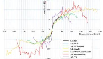
Figure 18: Ultimate load and ultimate lateral displacement obtained from pushover tests conducted in stone masonry walls with various strengthening options (Source: USAID/NSET, Baliyo Ghar Program)
