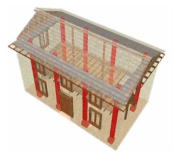
Figure 12: Position of strong backs (indicated in red) Figure 13: Slab strip (indicated in red) connects the in a house (Source: Build Change)
