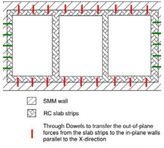
Through Dowels to transfer the out-of-plane forces from the slab strips to the in-plane walls parallel to the Y-direction
