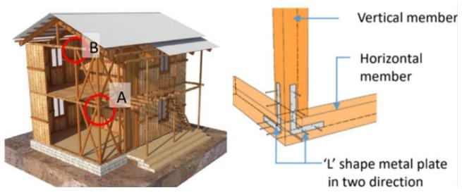
Figure 33: Schematic of timber house retrofit Figure 34: Detail at A: Connection at corners approach
