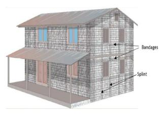
Figure 16: Schematic of splint and bandage Figure 17: Retrofit of a house using splint and bandage approach (Repair and retrofitting manual) (Source: NRA's Repair and Retrofitting Manual)
