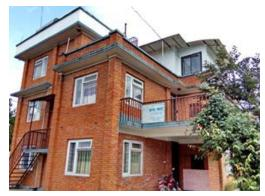
Figure 4: Typical brick in cement mortar house (Photo credit: Build Change)
