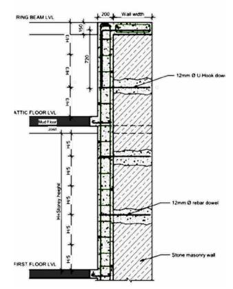
Figure 11: Detail of strong back installation
