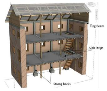
Figure 8: Schematic of strong back approach of retrofitting
