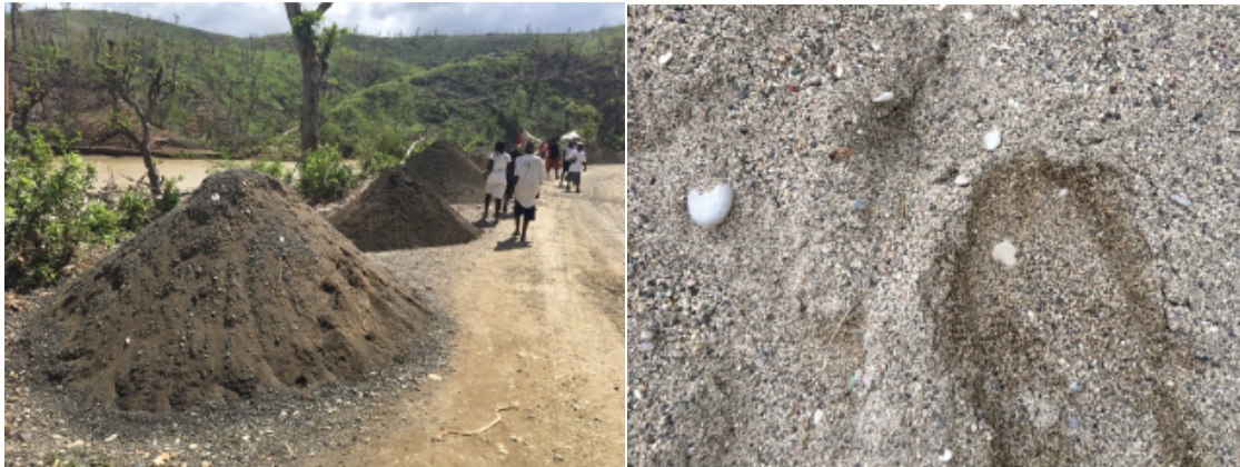
Figure 22 Left: River sand extracted from the riverbed, generally used unwashed. Right: Beach sand used for block manufacturing in Jérémie
