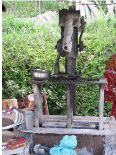
Figure 26. Concrete block hand press, Bahunepati.
