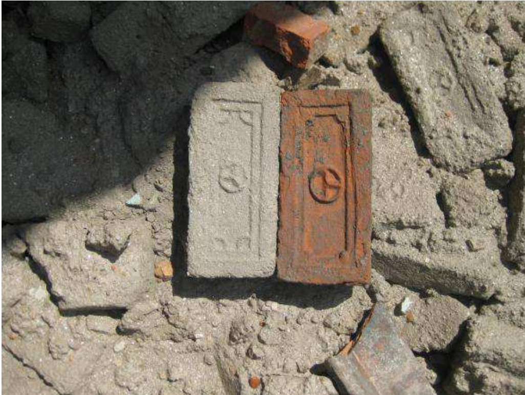
Figure 23 Unfired brick compared to fired brick
