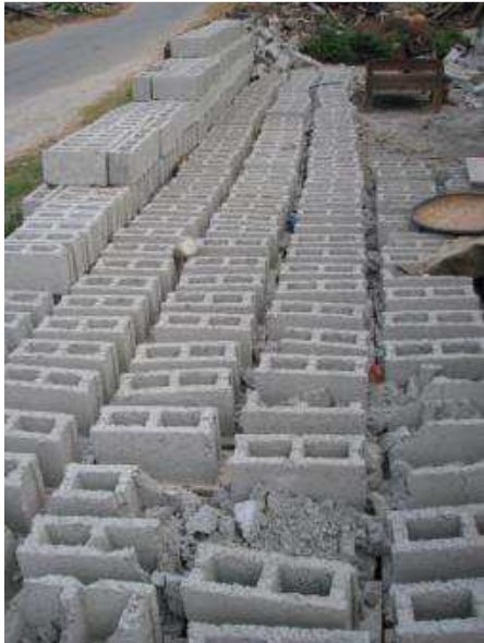
Figure 25. Handmade concrete blocks, Bahunepati.
