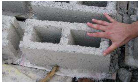
Figure 27. Handmade concrete block, curing, Bahunepati.
