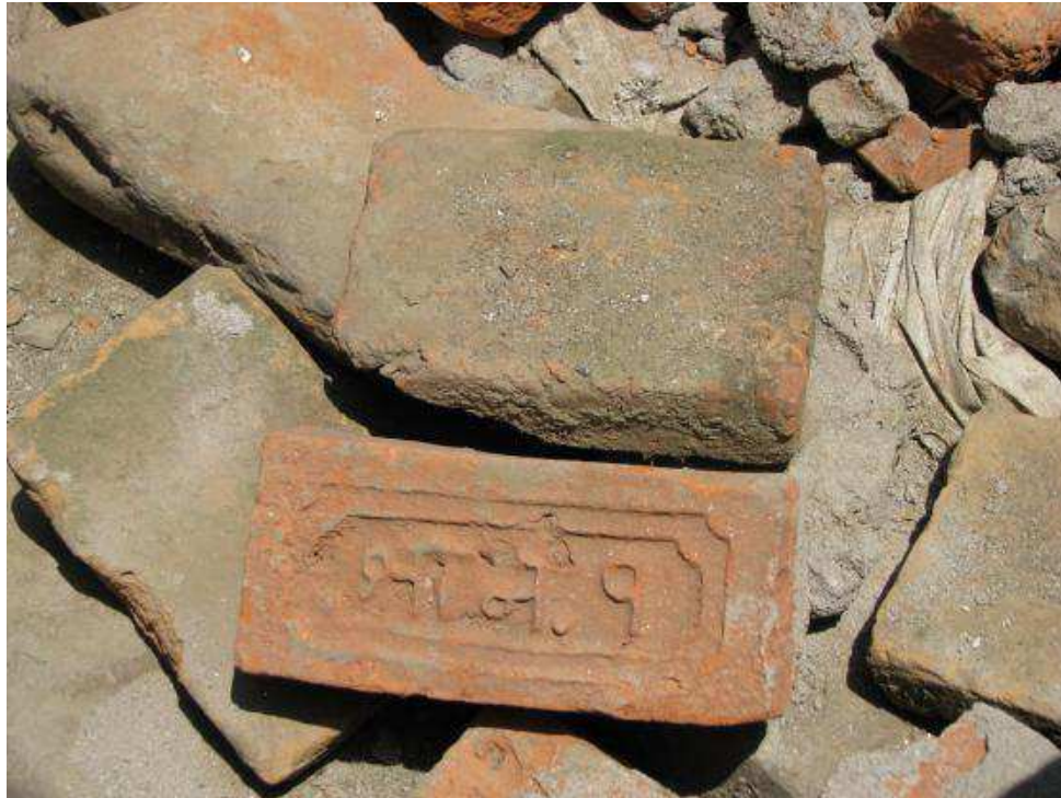
Figure 22. Older brick, above, compared to newer brick, below. Note brick maker's embossment on newer brick.
