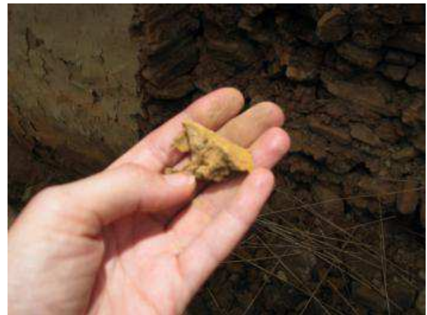
Figure 21. Piece of mud mortar, Thula Gaun.
