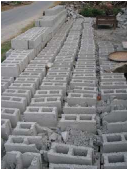
Figure 22. Handmade concrete blocks, Bahunepati.
