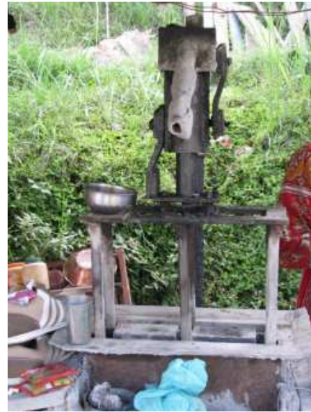
Figure 23. Concrete block hand press, Bahunepati.
