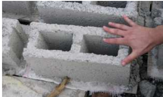
Figure 24. Handmade concrete block, curing, Bahunepati.
