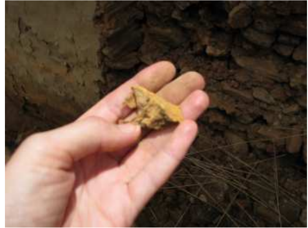
Figure 20. Piece of mud mortar, Thula Gaun.
