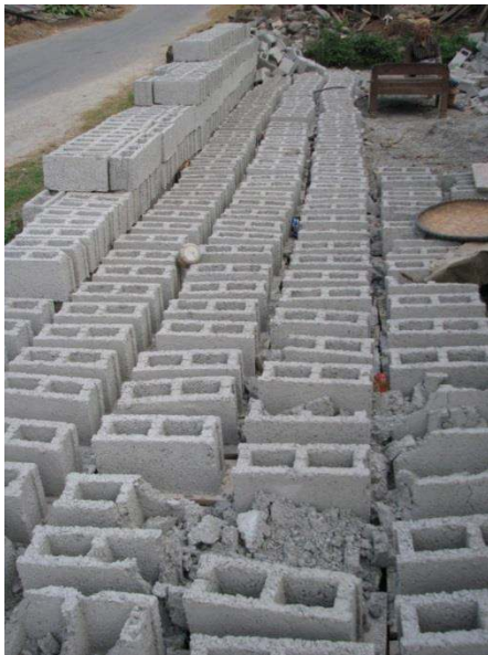
Figure 22. Handmade concrete blocks, Bahunepati.
