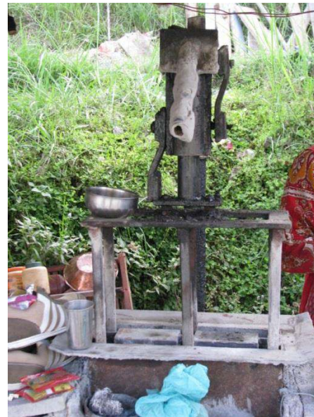
Figure 23. Concrete block hand press, Bahunepati.
