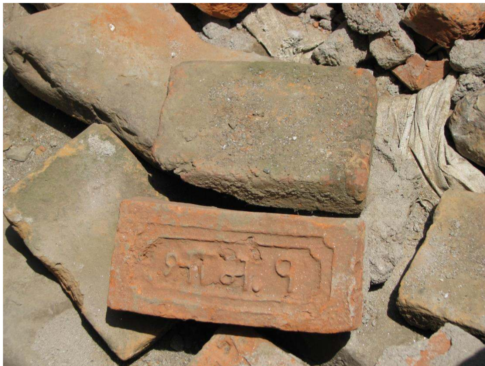
Figure 21. Older brick, above, compared to newer brick, below. Note brick maker's embossment on newer brick.
