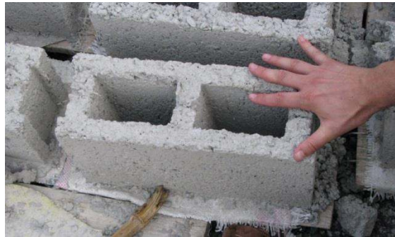
Figure 24. Handmade concrete block, curing, Bahunepati.
