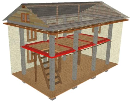
Fig. 17. Slab Strip (indicated in red) connects the diaphragm to the walls as well as interconnecting the strong backs
