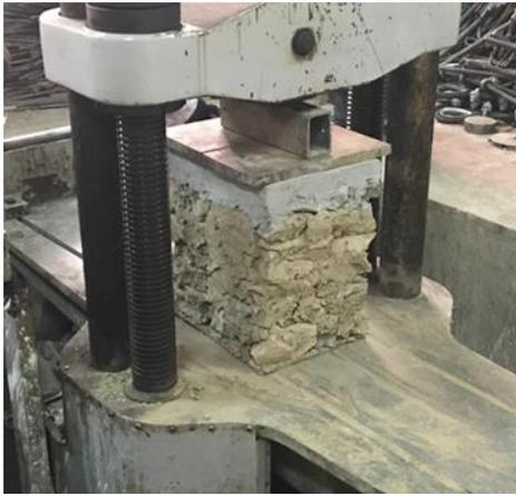
Fig. 20. Compressive test carried out
