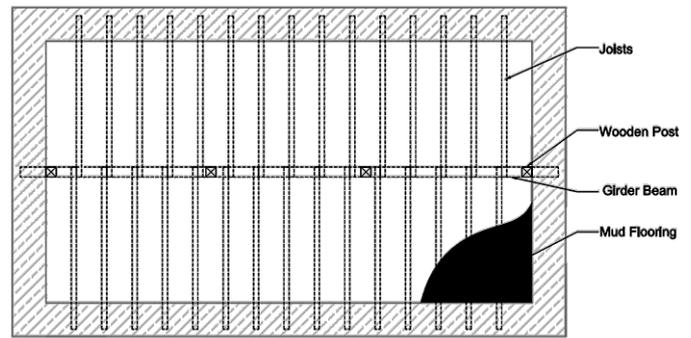
Fig. 6. Floor plan showing joist and Girder beam placements
