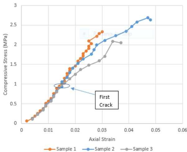
Fig. 21. Compressive stress vs Axial stress
