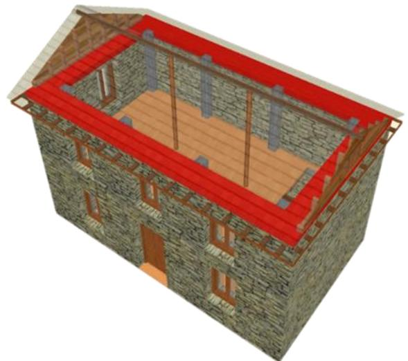
Fig. 14. Ring Beam highlighted in red is installed at the top of the attic wall
