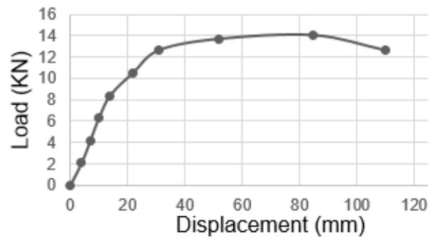
Fig. 22. load displacement curve for push out of dowels
